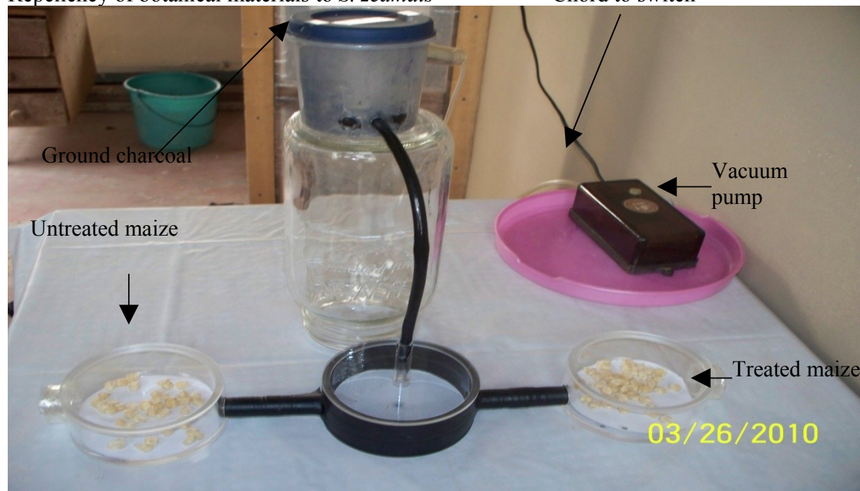
Plate 1: An olfactometer set up to study repellence of botanical extracts to S. zeamais (Courtesy Dr Haruna Braimah-CSIR-CRI)
