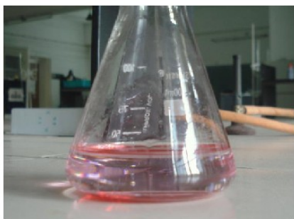
Figure 12: Red precipitate formed after adding conc. HCl
