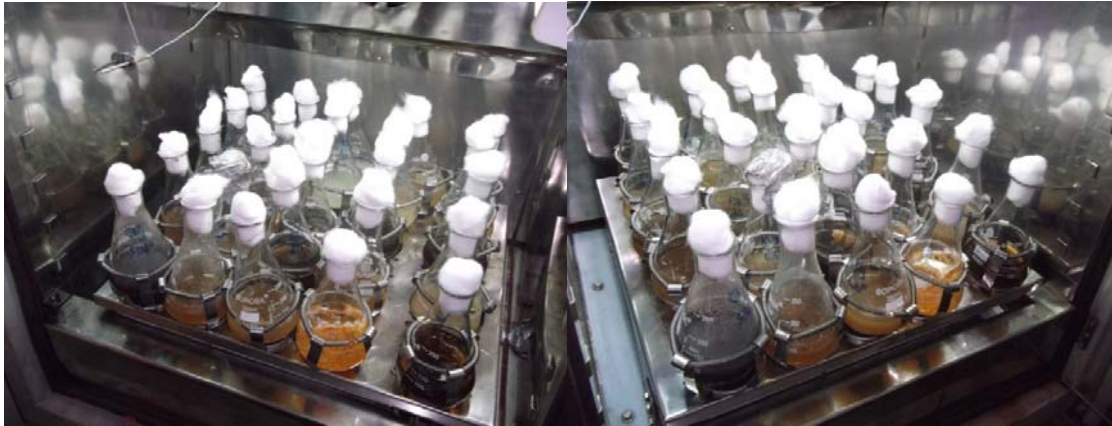
Fig1: Incubation of P. cinnabarinus in the production media at 120rpm for 15 days
