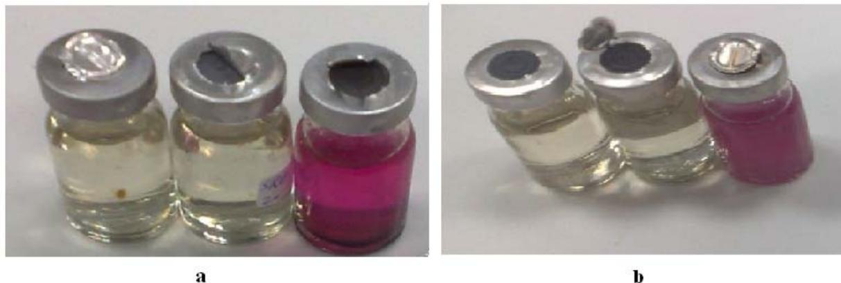
**Figure 10-a-SRB test is illustrated, in disinfection time with chlorine 0.5 mg/lit concentration and b-in disinfection time with ozone 0.1 mg/lit concentration**
