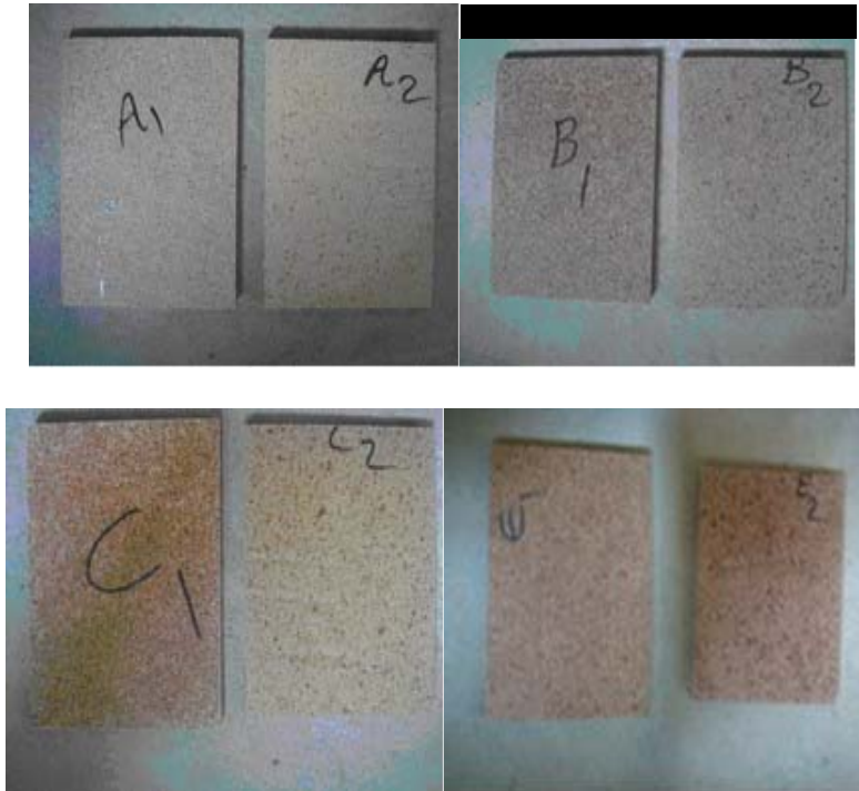
Figure-1. The boards produced from A. Fir wood B. Beech wood C. Poplar wood E. Alder wood with polyethylene using 1. Mesh 40 2. Mesh 80
