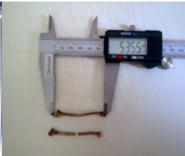
Figure 3: Measuring of tibia dimensions using digital caliper
