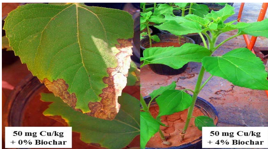
Figure 1. Effect of biochar application on copper toxicity in sunflower plant at 50 mg Cu/kg soil treatment (medium Cu toxicity)
