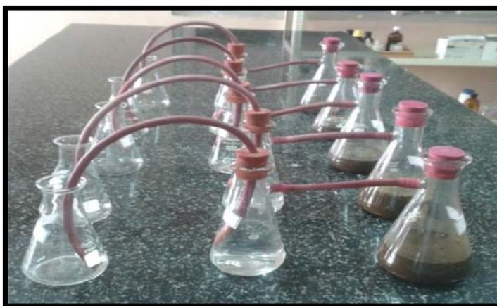
Fig: 1 Laboratory scale digester set-up
